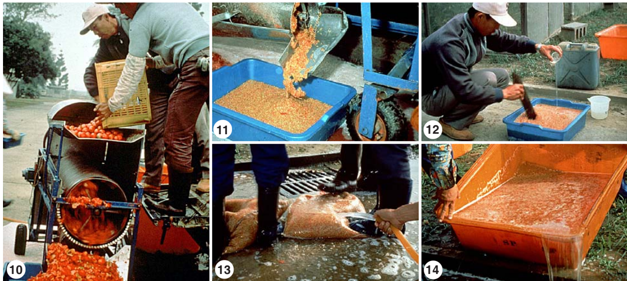
Figures 10-14. A machine extracts the seeds from fruits. Seeds are then treated with hydrochloric acid to loosen their gelatinous coating, and then cleaned using water.
